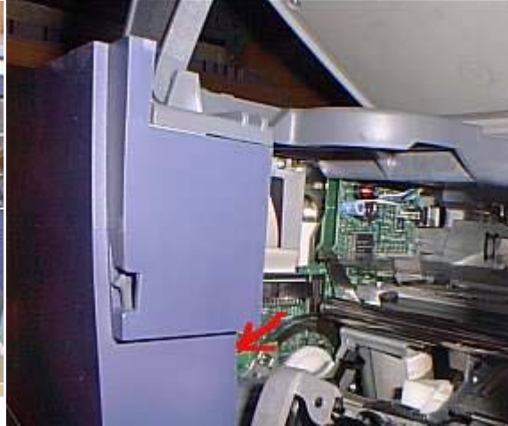
View looking toward left-inside. Red arrow points toward battery.
